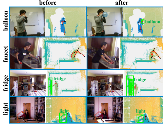
Figure 7. Human poses and depth images (before and after a fluent change) for actions as captured by the Kinect, together with sample frames.
